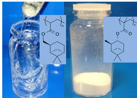
*Two of the terpene polymers we have created so far - very different glass transition temperatures are observed for the acrylates (left) and methacrylates (right) of  $\alpha$ -pinene*
