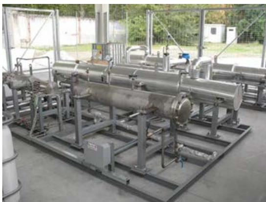
Figure 3: Pilot-scale unit for supercritical biodiesel production, designed and manufactured within the framework of the COPIRIDE FP7 EU project (CP-IP 228853)
